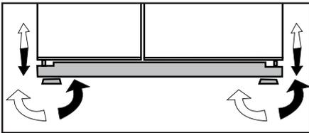
1. Remove the lower ventilation cover by unscrewing its screws as shown in the figure below. (See Figure B)
