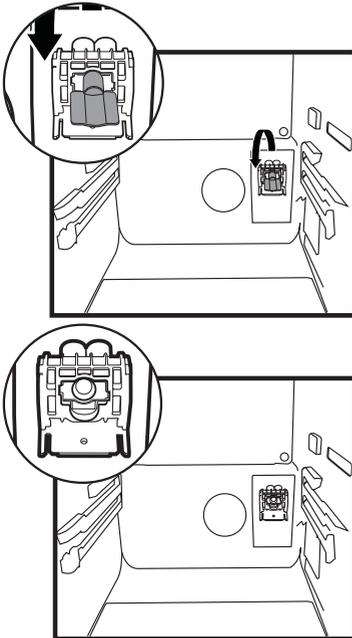
3. Take out the water filter by-pass cover by rotating it downwards. (Figure 3-4)
