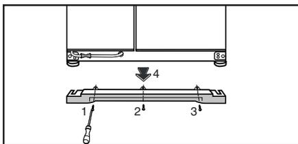
2. Loosen the three screws of the hinges of the lower door, which you wish to escalate, with the help of a screwdriver as shown in the figure below. (Do not remove completely) (See Figure C)
